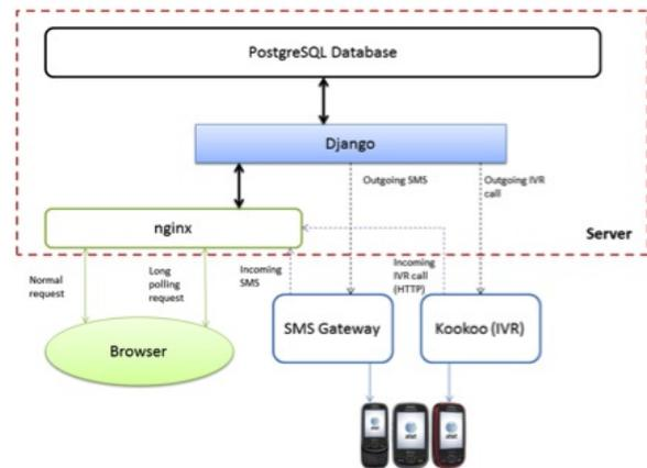
Figure 1: NextDrop System Architecture
